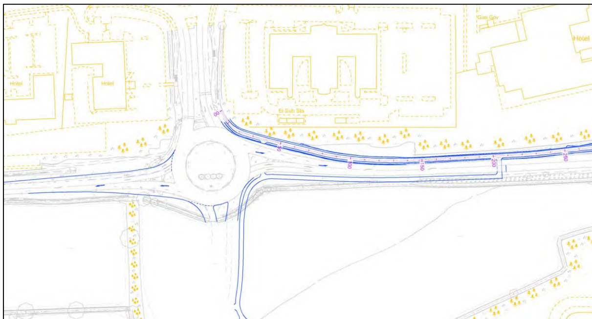
Figure 2.6: A453 EMGP2 Access Junction and Toucan Crossing
